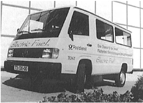
Fig. 2. German postal vehicle with zinc/air battery [2].
